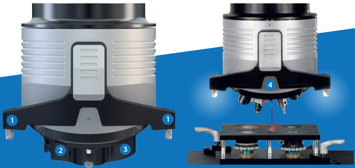
❶ POWER LED BANKS ❷ PROTECTION SKIRT ❸ 4 OBJECTIVES ❹ LASER POSITIONING SYSTEM
